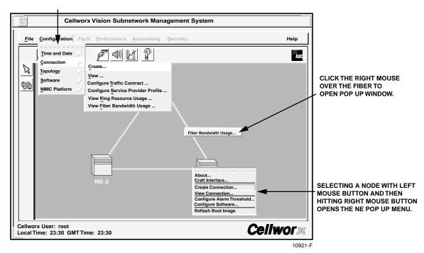
Figure 1-9. Cellworx STN GUI Display (sample)
